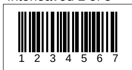
Interleaved 2 of 5 + CHECKSUM
